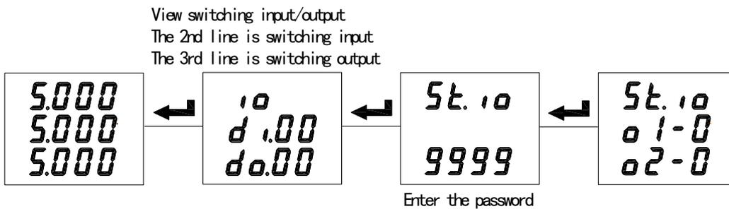
View the switching status of AMC72/96(L) single-phase current meter(same single-phase voltage meter):
