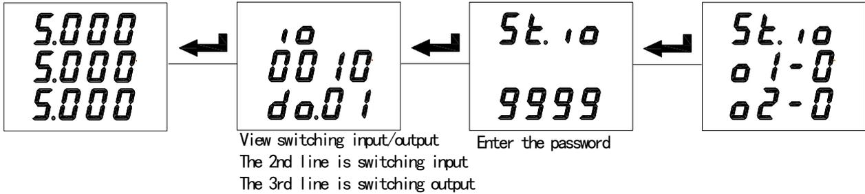
View the switching status of AMC72 (L) three-phase current meter (same three-phase voltage meter):
