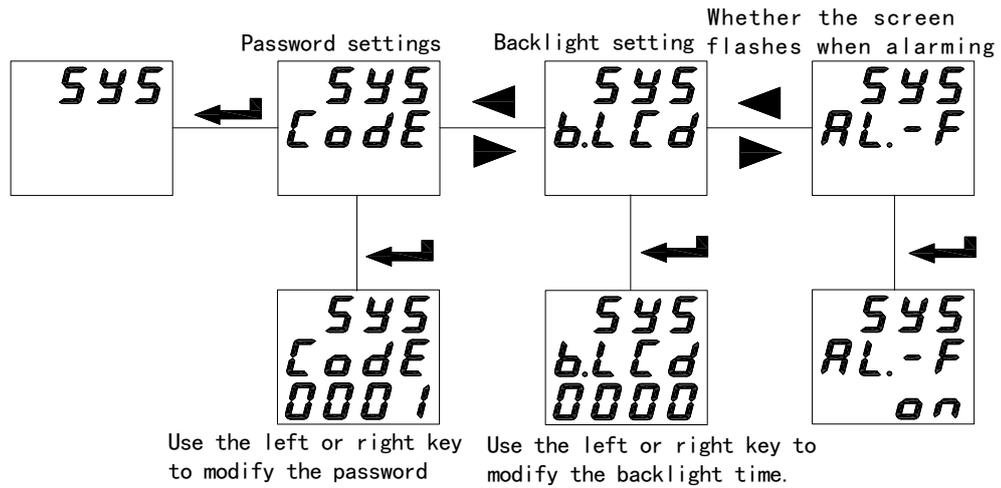
Enter the programming menu, press left or right key to select the LCD page, press Enter key to enter revising condition, left or right key to modify the time to 000 ~ 255s. To LED display meter, this item is invalid.
