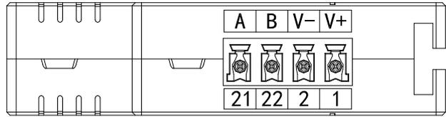
The function of the network port is the power interface and the RS485 interface. The specific definitions are as follows:
