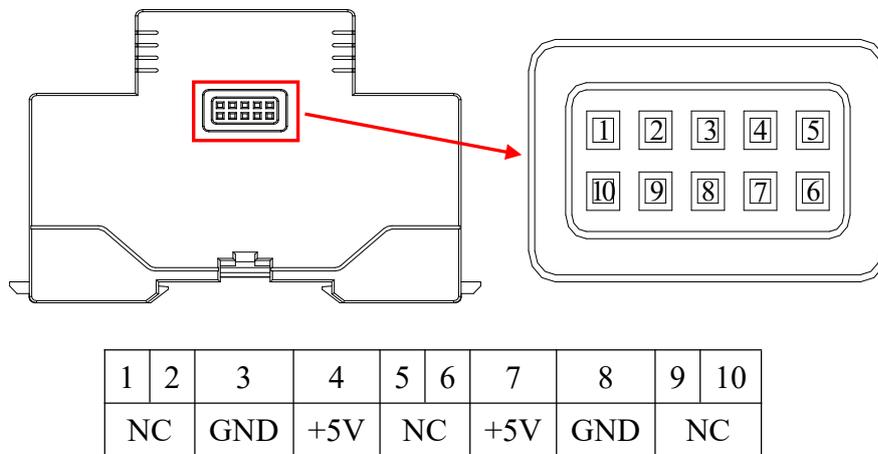
The side interface is used for the AWT100 wireless communication terminal to supply power through the AWT100-POW power module AC220V. The AWT100 wireless communication terminal is connected to the AWT100-POW power supply module through pins and fixed together by a buckle. The connection diagram is shown in Figure 4:
