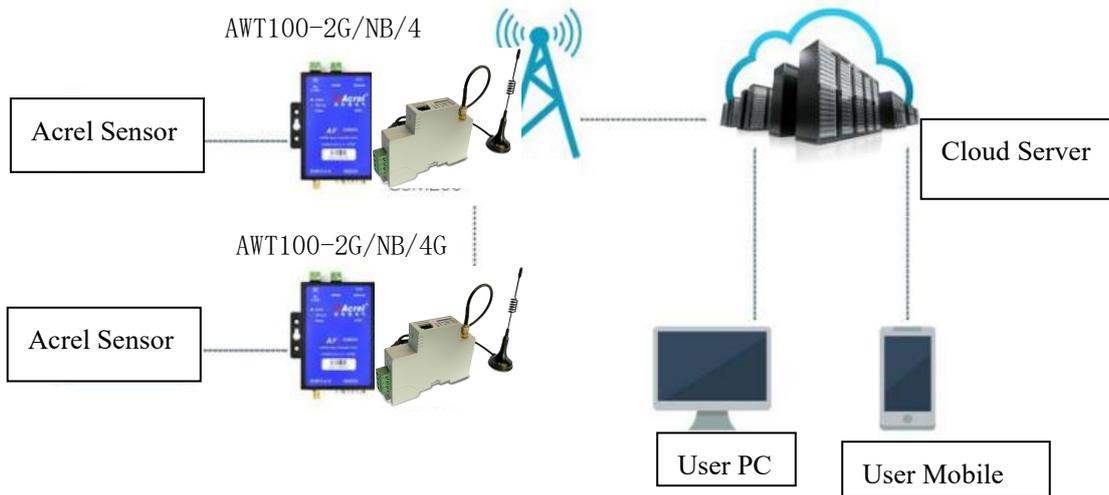
Figure 2 AWT100-2G/NB/4G Typical application of wireless communication terminal
