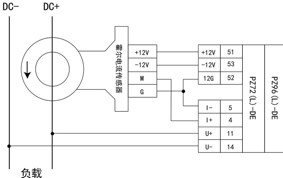
Figure 6 Typical wiring diagram of using Hall current sensor
