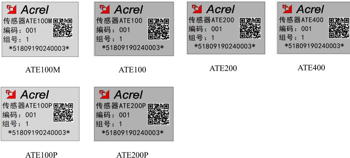
According to the above pictures, If the sensor is ATE100M/100/200/400/100P/200P, the group number of ATE must be same with the group number of ATC450-C/ATC600 and the installation order is base on the label. The code of each sensor is used to distinguish each sensor from same group. “**code: 001**” is recommended to be installed on the first temperature measuring point of the first cabinet, and then installed other sensors in this order.
