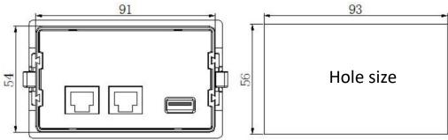
4) Temperature sensor (unit: mm)
