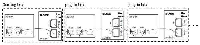
Connection of Detection Module with Display
