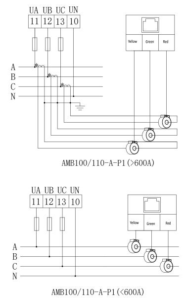
Note: The direction of current shall be as indicated by arrow on the transformer.
