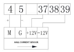
HALL SENSORS WITH ISOLATION FUNCTION WIRING
