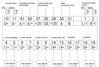
Note: arrow direction should be the same with current direction marked on the sensor .
